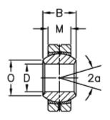
A = 18 a (degrees) = 13 B = 9 D = 6 Dynamic load C (kN) = 3.2M = 6.75
